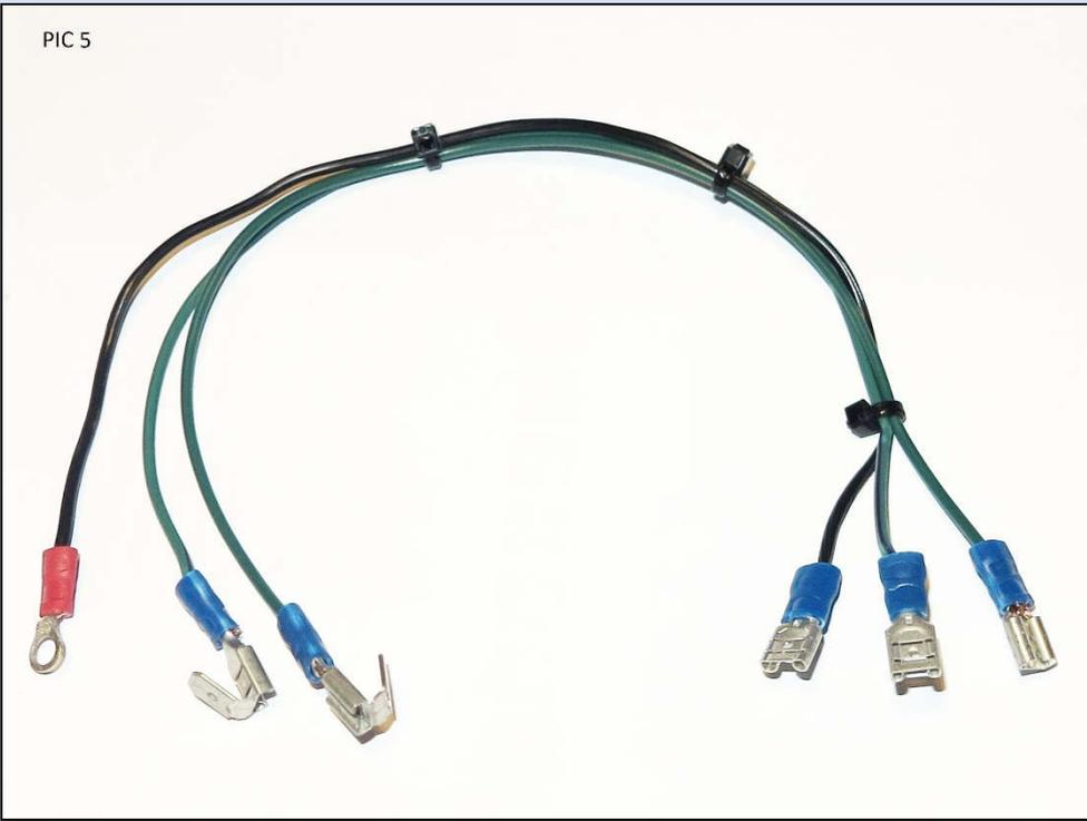
Connect the other three cables to the relay as per the circuit diagram, at the end of the article. Black to terminal 86, Green to terminal 85 and the green/Black cable to terminal 30.
